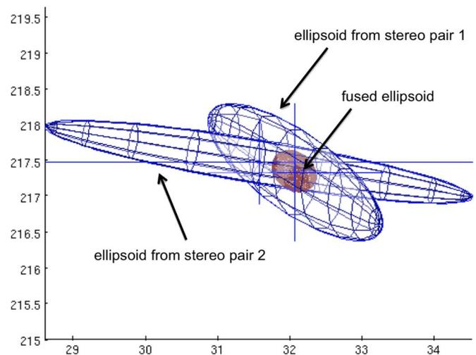
Fig. 5. Covariance ellipsoids of two corresponding points (obtained from the same marker) acquired by the two stereo pairs.
