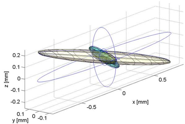
Fig. 8. Ellipsoids of the uncertainties obtained by the multi-stereo (the smaller one), multi-camera (the blue one), and single stereo approaches.
