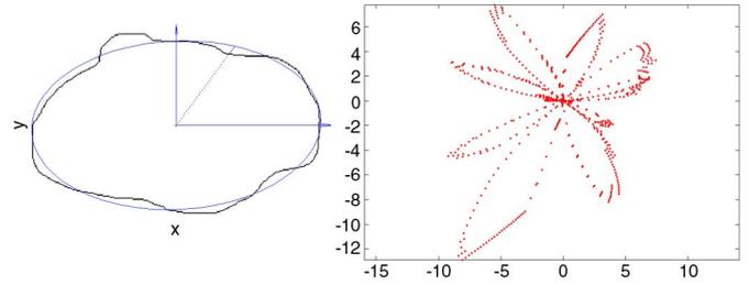
Fig. 1. Example of a badly segmented elliptical marker and the fitted one (on the left), and distribution  $\Delta_b$  (on the right).
