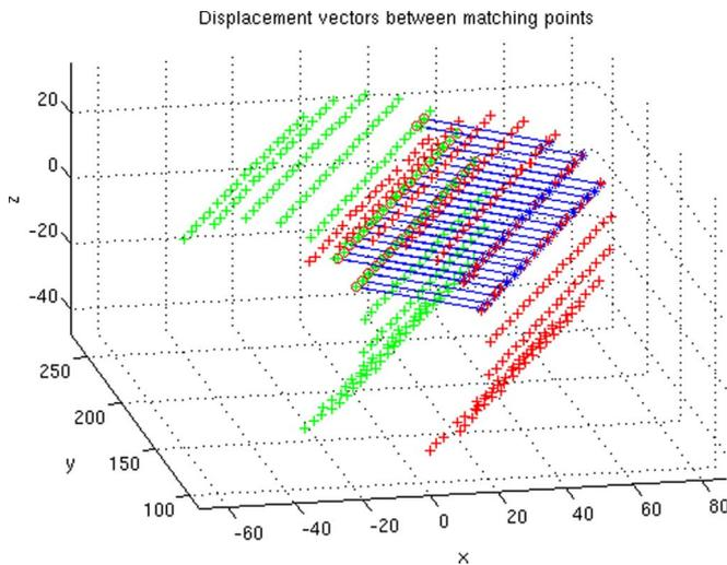
Fig. 7. Blue vectors show the estimated displacements of the matching points of A (green markers) and B (red markers).
