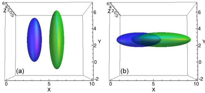
Fig. 2. Examples of different compatibility measures between the same couple of points, with the covariance ellipsoids of equal axis length but different orientation. In a) the MD is 4.5 and in b) the MD is 0.36.
